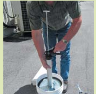
Ensure the tight seal, fully extend rod and fill the barrel. Disengage from the follow plate
